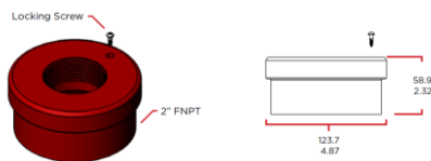
AD150JR ADAPTOR 2" JIC MALE X 2" NPT FEMALE WITH OPTIONAL INDICATOR **NOTE: RECEIVER IS SOLD SEPARATELY.
