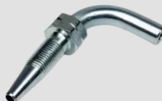
100-052 HOSE STUD 90° D 6 | H 13 | L 21 | HOSE Ø 4
