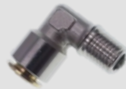
106-113 ; ELBOW QUICK CONNECTOR PIVOTABLE | D 6 | G M 10 X 1 TAP | SW 13
