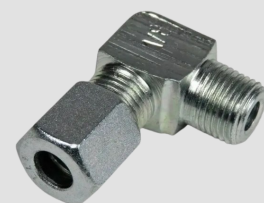
106-103 ; ELBOW MALE SCREW-IN FITTING | LL | D 6 | G 10 X 1 TAP | SW 11 | SW1 12
