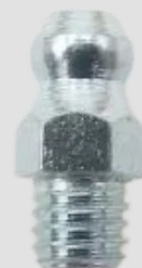
250-004, GREASE NIPPLE G R 1/8 BSPT H 1 DIN 71412 A
