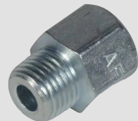
2510-106; ADAPTER - EXTENSION-PIECE | G M 10 X 1 TAP | G 1 RP 1/8 BSP L L 18 | SW 13
