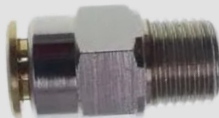
106-053 ; QUICK CONNECTOR STRAIGHT | D 6 | G M 10 X 1 TAP | SW 12
