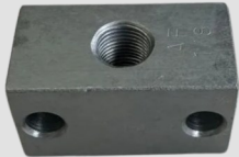
5029-111; GREASING BLOCK GG 1/8 BSP | D 2 x 6,5 | 20x20
