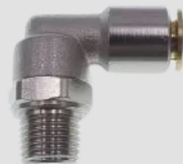
106-115-UNF ELBOW QUICK CONNECTOR PIVOTABLE D 6 | G 1/4 - 28 UNF | SW 13
