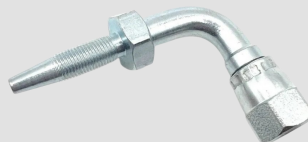
SE-STJIC908.6SS; STAINLESS 90 DEG 7/16 JIC REUSABLE HOSE END FOR 8.6; JIC FEM 90DEG DN4 HOSE (1PC) 4.1 ID
