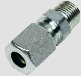
106-004-NPT ; STRAIGHT MALE SCREW-IN FITTING | LL | D 6 | G 1/8 NPT | SW 11 | SW1 12
