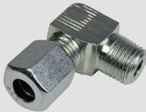
106-104; ELBOW MALE SCREW-IN FITTING | LL | D 6 | G R 1/8 BSP TAP | SW 11 | SW 1 12
