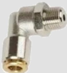
106-114 ; ELBOW QUICK CONNECTOR PIVOTABLE | D 6 | G R 1/8 BSP TAP | SW 13
