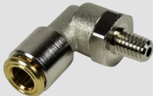
106-111 ; ELBOW QUICK CONNECTOR PIVOTABLE | D 6 | G M 6 X 1 TAP | SW 13
