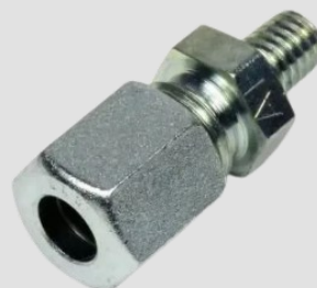
106-001 ; STRAIGHT MALE SCREW-IN FITTING | LL | D 6 | G M 6 X 1 TAP | SW 11 | SW1 12
